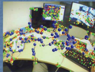
Tracking using the PTAM algorithm. Real-world feature points are used in conjunction with the SLAM concept. (Photograph courtesy Georg Klein and David Murray, University of Oxford)
