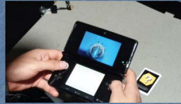
A lenticular display. (Photograph courtesy of Joseph J. LaViola Jr.)
