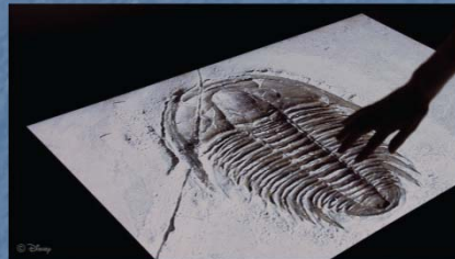
Electrovibration displays allow the user to feel the bumps and ridges on the 3D rendering projected on the surface of the display. (Photograph courtesy of Ivan Poupyrev, copyright Disney, printed with permission)
