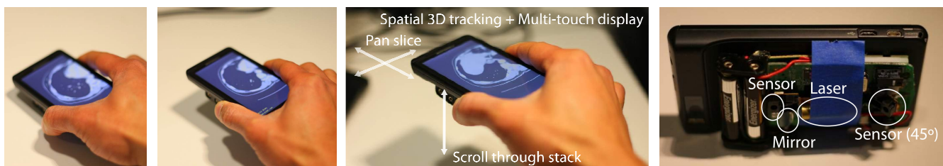
Figure 13: The Mobile Viewport adds relative 3D tracking to a mobile phone. Interaction is supported both by moving the device in 3D space and through multi-touch interaction on the display. A user can pan around in a medical image viewer and scroll through a CT stack by moving the device in 3D, or pan around in the view of a web page and control zoom level with distance.
