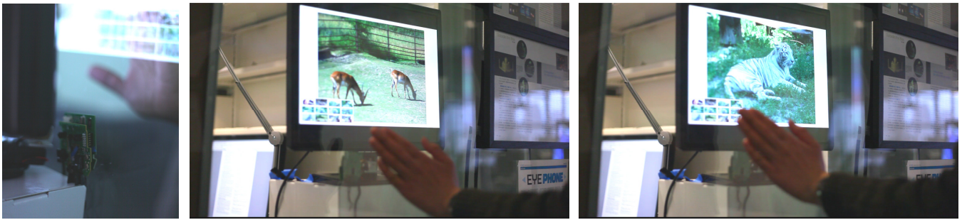
Figure 14. Low-cost motion tracking for public displays using an embedded Speckle projector and sensor (configuration D). The user's 2D hand movement selects the fullscreen image from a matrix of thumbnails in the lower left corner.
