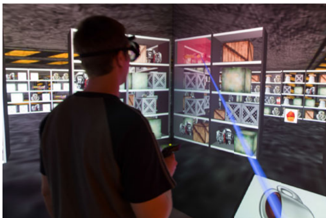
Fig. 1. A user selecting a target object on a shelf in the maze-like virtual environment used for the experiment.
