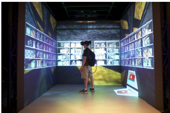
Fig. 2. This figure shows a user in the 270 degree CAVE while wearing the HMD setup. In the study, users only used one display at a time.
