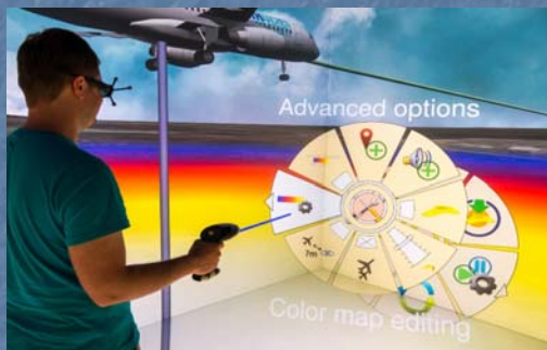
Pie menu in immersive virtual environment. (Photograph courtesy of Thorsten Kühlen, Virtual Reality & Immersive Visualization Group, RWTH Aachen)
