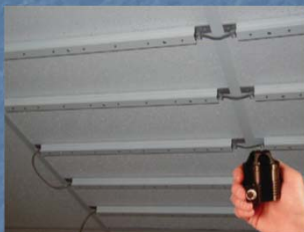
Marker-based inside-out tracking system with active LED beacons mounted on the ceiling and the camera sensors located in a handheld object. (Photograph of the HiBall-3000 Tracker courtesy of 3rd Tech, Inc.)
