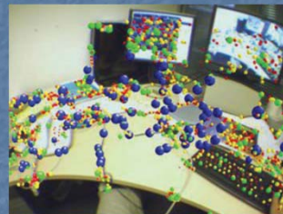
Tracking using the PTAM algorithm. Real-world feature points are used in conjunction with the SLAM concept. (Photograph courtesy Georg Klein and David Murray, University of Oxford)
