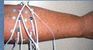
An example of EMG sensors applied to a user's forearm. (Photograph courtesy of Desney Tan, Microsoft Research)
