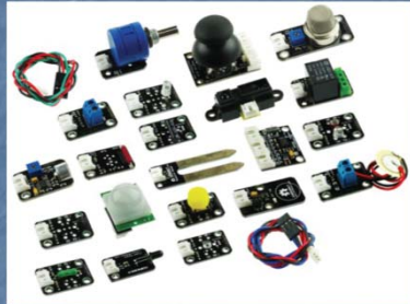
A variety of different sensors that can be used to for DIY input devices. The image shows light, sound, distance, magnetic, accelerometer, vibration, touch, and gas sensors. (Photograph courtesy of RobotShop, Inc.)
