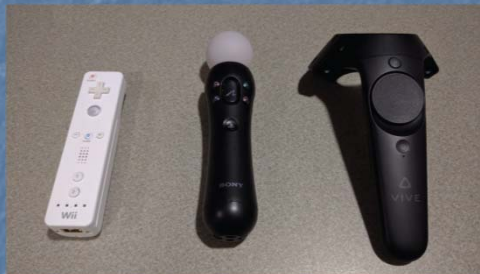
Examples of modern 3D mice that make use of optical and inertial sensing to produce 3D position, orientation, and motion data. Since users hold a 3D mouse, their hands are effectively tracked in 3D space, and coupled with buttons, analog controllers, dials, etc., these 3D mice provide for a variety of mappings from device to 3D interaction technique. (Photograph courtesy of Joseph J. LaViola Jr.)
