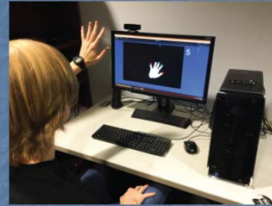
Example of tracking the fingers using a depth camera, making use of passive sensing (Photograph courtesy of Arun Kulshreshth)
