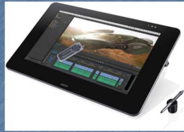
A large pen- and touch-based LCD tablet allowing the user to draw directly on the screen. (Photograph courtesy of Wacom Technology)
