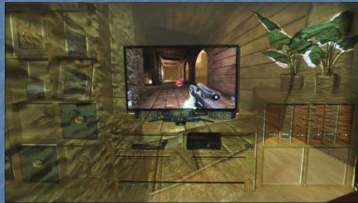
The Illumroom, an example of projection mapping to create an extended display in a living room. The projector-camera pair correctly projects onto the various surfaces in the room. (Photograph courtesy of Microsoft)
