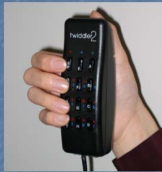
A 12-key chord keyboard (Photograph courtesy of Doug Bowman)
