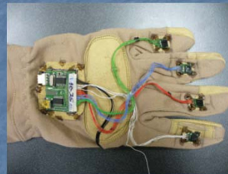
A data glove that uses accelerometers, gyroscopes, and magnetometers to capture information about each finger. (NuGlove Photograph courtesy of AnthroTronix)
