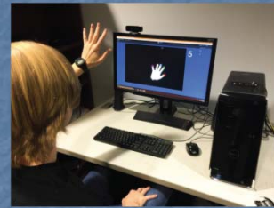
Example of tracking the fingers using a depth camera, making use of passive sensing (Photograph courtesy of Arun Kulshreshth)
