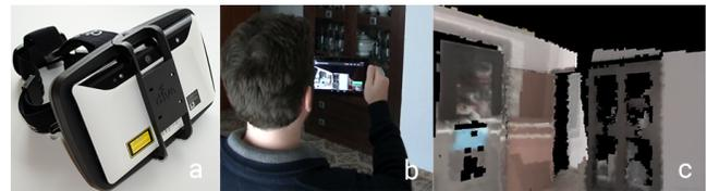
**Figure 3:** (a) Tango in a virtual reality headset. (b) A user walking with the Tango device to create a 3D model of a room. (c) The generated 3D model. Scanning a  $3 \times 4$  m full room took less than 3 minutes.
