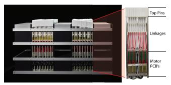
Figure 13. Side view of the TRANSFORM system with a single 12x2 actuation module.
