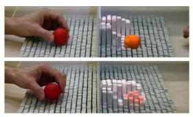
Figure 3. Top: Two linked tangible tokens at two locations, with synchronized position. Bottom: A tangible token rendered with the shape display at a remote location.
