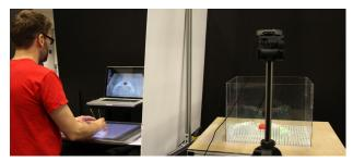
Figure 16. Setup of the telemanipulation study. Left: The participant's gestures are captured and two screens provide visual feedback. Right: Shape output moves the target ball.
