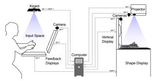
Figure 14. System diagram of the telemanipulation system using shape capture and remore shape display.
