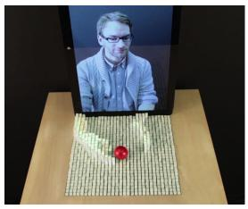
Figure 2. A user manipulating a sphere through his remote physical embodiment.
