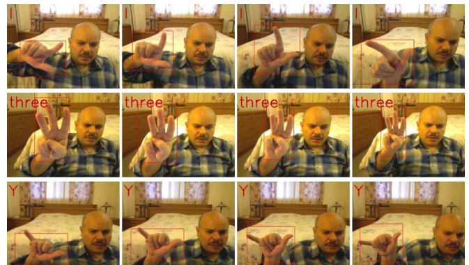
Fig. 16. Hand gesture detection and recognition for I (L), W (three), and Y postures.
