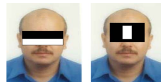
Fig. 8. Detecting a human face using Haar-like features.
