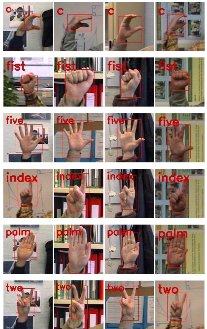
Fig. 18. Hand posture detection and recognition for the six hand postures of Marcel database images using our approach.
