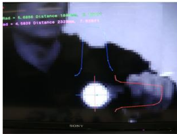
Figure 21: Visualizing the 2D pixel intensity distribution of the PlayStation Move sphere is useful for debugging the model fitting stage.
