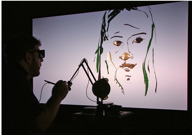
Figure 12: The haptic-based Drawing on Air 3D interface.
