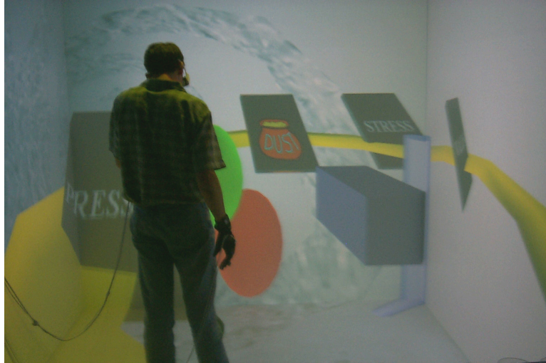
Figure 9: An example of a virtual toolbelt. The user looks down to invoke the belt and can grab tools and use them in the virtual environment.
