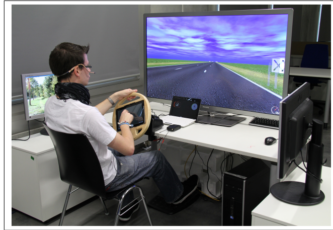
Figure 1.10 Multimodal automobile interface combining speech with gestures on the steering wheel. Reproduced by permission of Bastian Pfleging.
