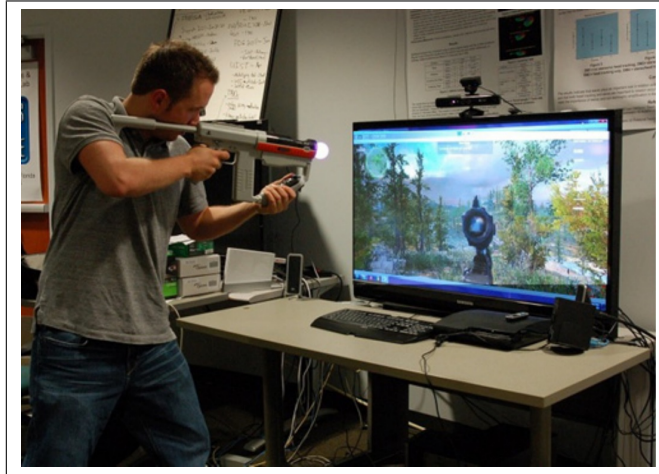
Figure 1.11 RealEdge prototype with Kinect and PS Move Controller. Reproduced by permission of Brian Williamson.
