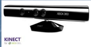
Xbox 360 Kinect Structured Light
