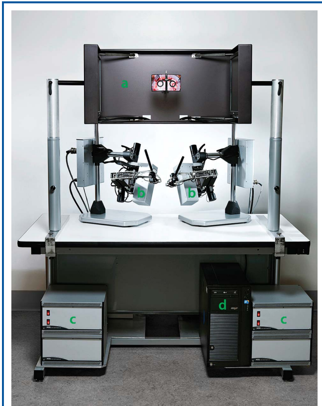
FIGURE 2. NeuroTouch components. Stereoscope (a), haptic systems (b), power supplies and amplifiers for haptic systems (c), computer (d).
