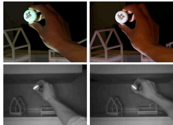
Figure 10. As the user tilts the outer plastic layer, the system senses the orientation and updates the projected images, while the spherical magnet stays in the same orientation.
