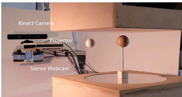
Figure 8. Tracking and Projection System of ZeroN.
