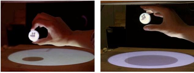
Figure 13. The size of digital shadow is mapped to the height of ZeroN.
