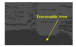
Figure 4: Log-Filtered Gradient of 3D Depth Image; Solid Dark Gray Patch Indicates Flat Traversable Region of Image (Indicated in Yellow)
