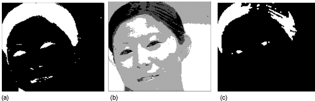
Fig. 5 – Pupils identification. (a) Image mask selecting the darkest elements in the early four levels segmentation in Fig. 4c; (b) final four levels segmentation where the pupils are separated from the sclera; (c) darkest elements of (b).
