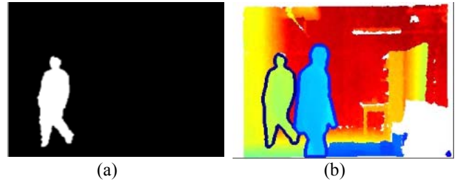
Fig. 7. (a) Result of our region growing algorithm. (b) The extracted whole body contours are superimposed on the depth map.
