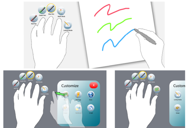
Figure 11. Placing palm and fingers on surface activates PalmPrint menu. Lifting and tapping a finger changes the pen mode. Chording is also possible. A Customize palette allows drag and remapping of functions.
