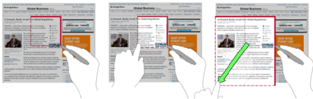
Figure 9. Drawing a crop marks displays a feedforward selection/clipping marquee widget. Dragging the marquee while drawing switches to bi-manual rectangular selection.
