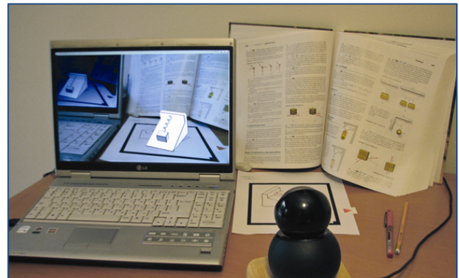
Figure 7. System Setup. An inclined plane, a box, and a spring are augmented on top of their sketch. The setup consists of paper, a pencil, a red pen, and a computer connected to a webcam.
