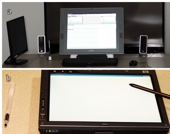
Figure 1: The wizard station (a) is composed of a desktop PC and two monitors, a 21" monitor (center) and a 17" monitor (left). The recognition station (b) is a tablet PC.
