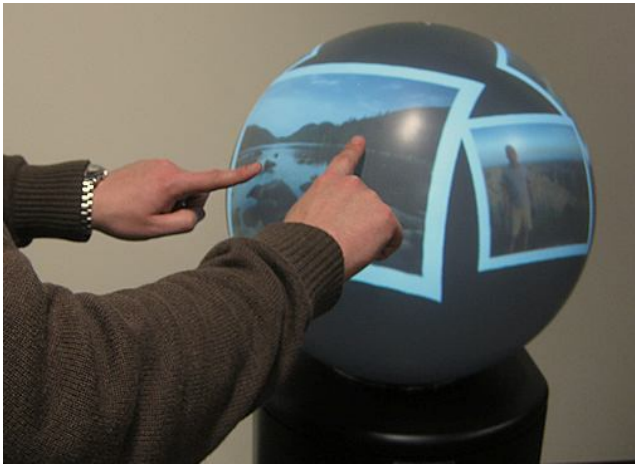
Figure 6: Interacting with a picture on Sphere, a multi-user, multi-touch spherical display prototype built on top of Global Imagination’s Magic Planet display.
