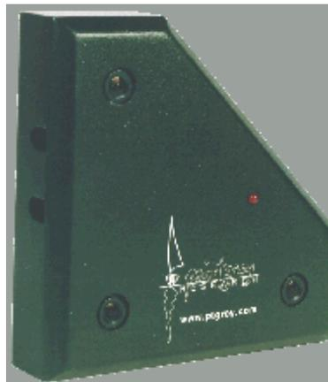
Figure 5.2: The Digiclops stereo system
