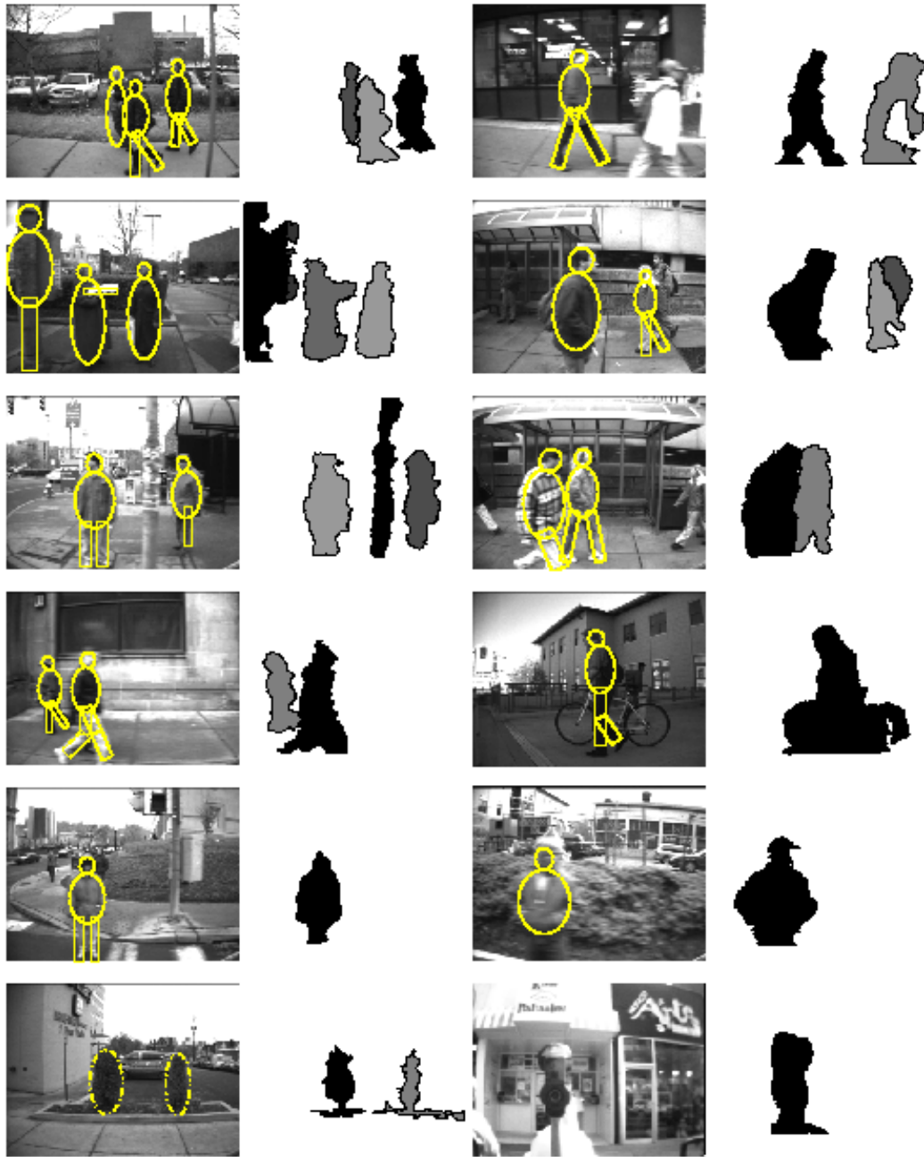
Figure 5.3: Sample results of pedestrian detection ( the unidentified objects are circled by dotted lines)
