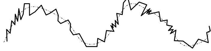
This signal can be <u>decomposed</u> into two signals (long term and short term), each can be simulated by an appropriate model.
