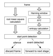
Figure 3: Work flow of the preprocessing component
