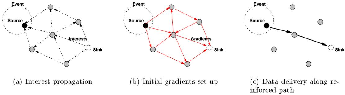
Figure 1: A simplified schematic for directed diffusion.
