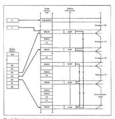
Fig. 5. Display registers indicating current addressing environment.
