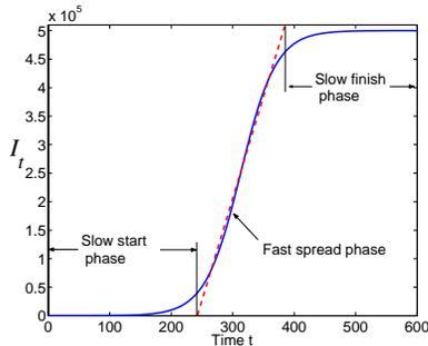
Figure 1: Worm propagation model
