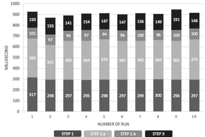
Fig. 6. Execution time performance results of each step in the secure backup procedure on a smart card in ten test runs
