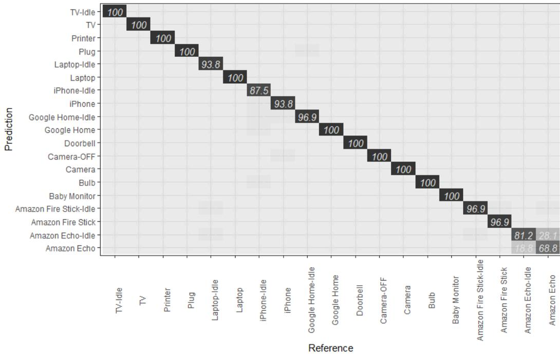
Fig. 7. Confusion matrix of our IoT devices classification based on summary dataset using RF machine learning algorithm.
