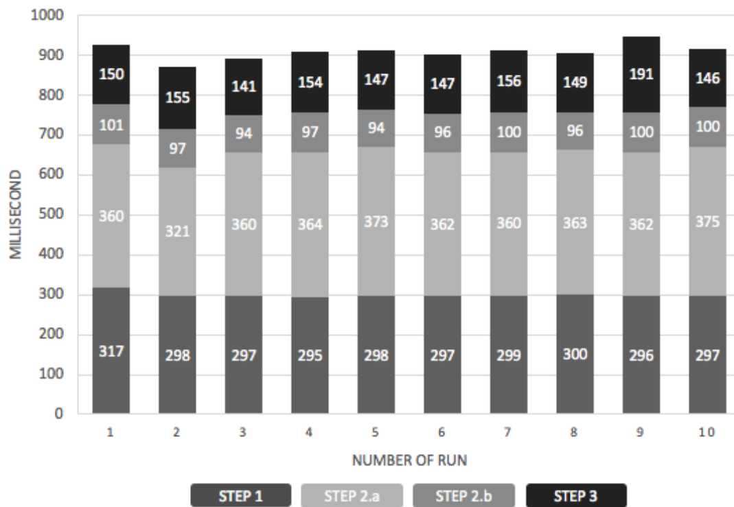
Figure 3-7: Performance results of the secure backup procedure on a smart card
