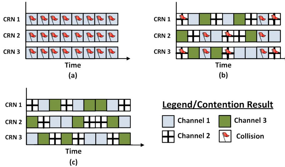
Figure 2: Channel access pattern of CRNs. (a) Selfish behavior from CRNs for best quality channel (channel 1) will always result in a collision. (b) Fair distribution of spectrum resource when CRNs mix their choice of channels according to MSNE. However, MSNE is inefficient because of collisions and wasted opportunities. (c) Fair and efficient resource distribution with CE.
