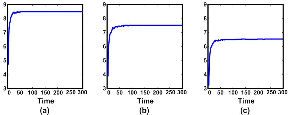
Figure 9: Comparison of CE values when channel payoffs (quality of channels) are varied. Y-axes represent expected utility per CRN with  $k = n = 3$ , (a)  $u_1 = 9, u_2 = 8, u_3 = 7$ , (b)  $u_1 = 9, u_2 = 8, u_3 = 4$  and (c)  $u_1 = 9, u_2 = 8, u_3 = 1$  Decrease in the quality of channel 3 results in a proportional decrease in the expected utility for every CRN. Also, the convergence rate decreases as the variance in channel quality increases.
