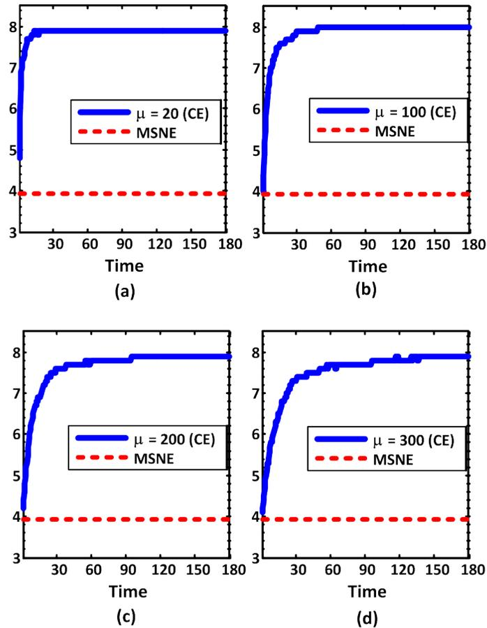
Figure 3: Expected utilities per CRN for  $N = 2, K = 2$  and utilities from the two channels are:  $u_1 = 9$  and  $u_2 = 7$  with varying inertia parameter  $\mu$ . (a)  $\mu = 20$ , (b)  $\mu = 100$ , (c)  $\mu = 200$  and (d)  $\mu = 300$ . Different values of  $\mu$  achieve the same convergence value of expected utility however as inertia increases, it causes a decrease in convergence rate.
