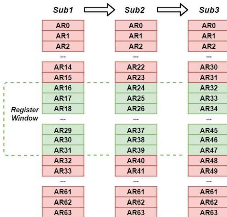
Figure 4.1: Overview of the ESP32 register file and register window mechanism. A function only has access to the registers contained in the register window.
