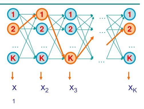
$$\begin{split} P(x,\pi) &= P(x_1,\,...,\,x_N,\,\pi_1,\,.....,\,\pi_N) = \\ &P(x_N,\,\pi_N \mid \pi_{N-1}) \; P(x_{N-1},\,\pi_{N-1} \mid \pi_{N-2}).....P(x_2,\,\pi_2 \mid \pi_1) \; P(x_1,\,\pi_1) = \\ &P(x_N \mid \pi_N) \; P(\pi_N \mid \pi_{N-1}) \; .....P(x_2 \mid \pi_2) \; P(\pi_2 \mid \pi_1) \; P(x_1 \mid \pi_1) \; P(\pi_1) = \\ &a_{0\pi 1} \, a_{\pi 1\pi 2}.....a_{\pi N-1\pi N} \; e_{\pi 1}(x_1).....e_{\pi N}(x_N) \end{split}$$
