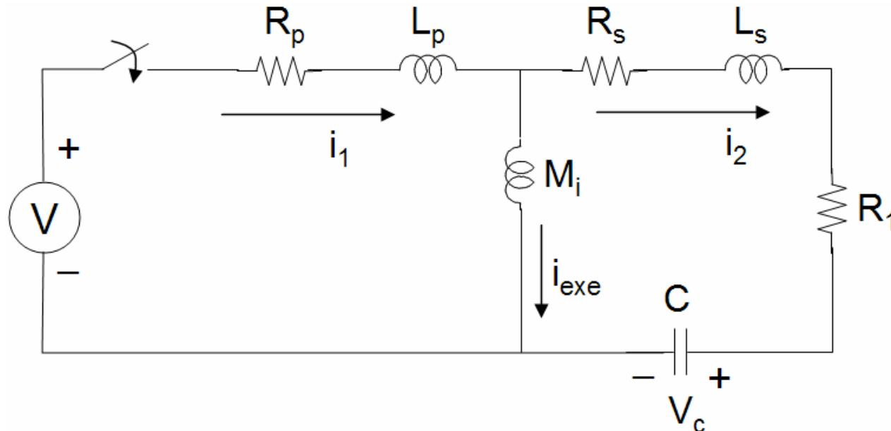
where:  $L_p = 0.1 \text{ H}$ ,  $L_s = 0.2 \text{ H}$ ,  $R_p = 1 \Omega$ ,  $R_s = 2 \Omega$ ,  $R_1 = 1 \Omega$ ,  $M_i = 0.1 \text{ H}$ ,  $C = 1 \mu\text{F}$ , and  $V = 10 \text{ V}$  (Step Input)
