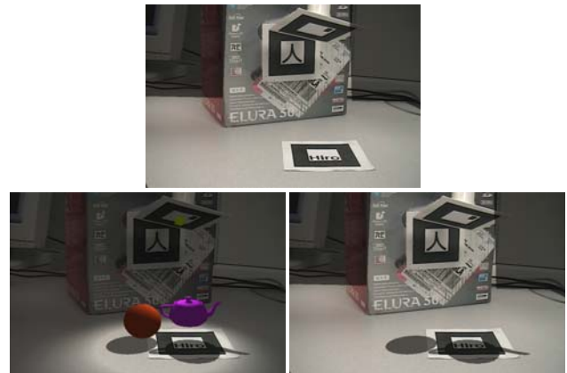
Figure 7. Sequence of virtual flashlight illuminating a real scene, clockwise from top: (a) Original intensity, (b) virtual-to-real shadowing, (d) lit virtual and real objects with shadow in a darkened surrounding.
