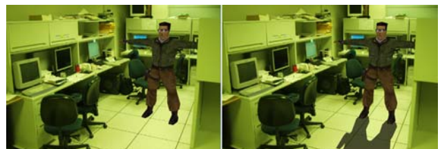
Figure 4. A real scene with and without shadow cast from the virtual object.
