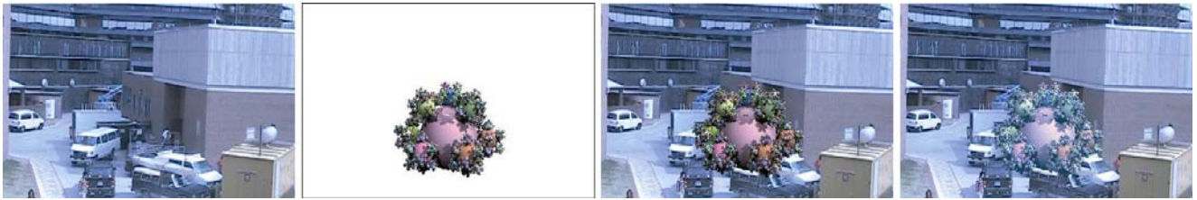
Figure 1. Video frame, rendered frame, result of compositing, and result of color adjustment algorithm.
