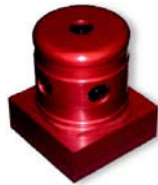
Figure 3. The Ladybug camera for real-time capture of environment light. Details about the camera and its capabilities can be found from Pointgrey Research ( http://www.ptgrey.com/products/ladybug ).
