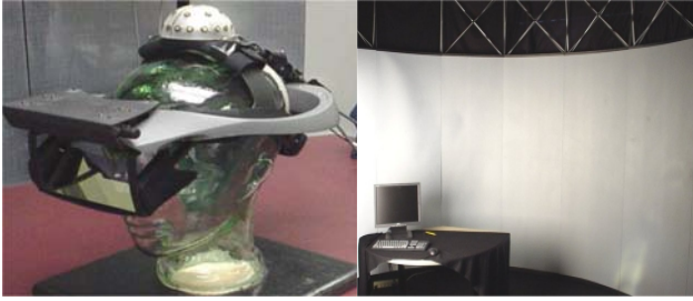
(a) Optical See-through HMD (b) ARC Display Fig. 6 Hardware components
