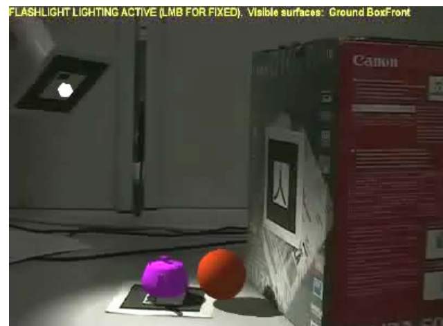
Figure 3. Virtual flashlight illuminating virtual/real objects
